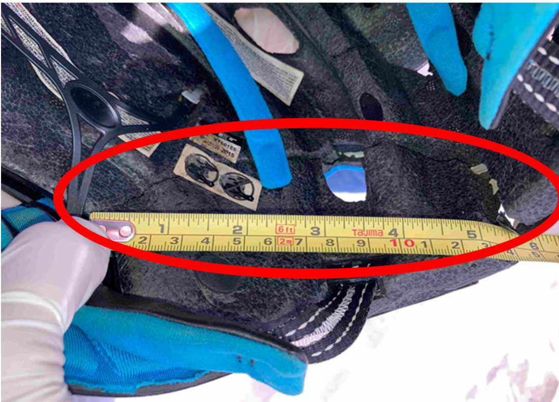
Figure 31: Damage on the Right-hand Side of the Helmet (Inner View)
