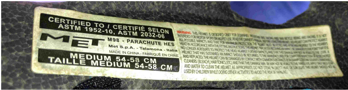
Figure 27: The Model and Certification Label of the Helmet
