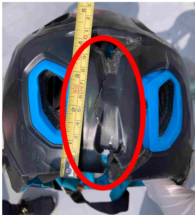
Figure 29: Damage on the Backside of the Helmet (Outer View)
